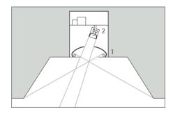
Custom designed luminaire based on a standard product: the optical system of a conventional louvred luminaire (below) is used as the direct ele-ment within a linear secondary reflector luminaire (above).
